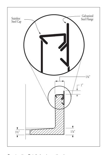
Construction Detail showing optional flange and cap.
